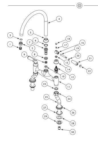
The set comprises of the following: ITEM QTY DESCRIPTION Aerator 2 Aerator Housing O-Ring 4 Spout Spout Cover Spout Bushing Connector 8 Connector Bushing 9 O-Ring 2 10 Connector Ring П Mixer RTC Valve 12 LTC Valve 13 14 Valve Cover 15 Handle Ring 2 16 2 Handle 17 2 Screw 18 2 Indicie 19 2 Handle Stem 20 2 O-Ring 21 2 Ceramic Handle 22 2 Ceramic Handle Nut 23 2 Sealing Washer 24 2 Nut 25 2 Leg 26 2 Plate 27 2 O-Ring 28 2 Washer 29 2 Nut 30 2 Non-return Valve
