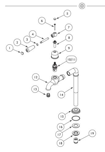
1 2 Ceramic Handle Nut 2 2 Ceramic Handle 3 2 O-Ring 4 2 Handle Stem 5 2 Indicie 6 2 Screw Handle 7 2 8 2 Handle extension 9 2 Valve Cover 10 LTC Ceramic Valve RTC Ceramic Valve 11 12 2 Tap Body
