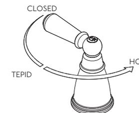
The side spray uses a sequential cartridge. This means that you will have cold, tepid and hot water, in this order, once you start opening the tap
