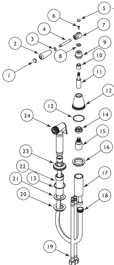
**Please Note:** This item can be carefully prised off with a sharp implement. The securing bolt for the handle can then be accessed and easily removed or tightened using a small allen key.
