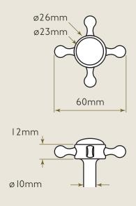
RECOMMENDED HOLE SIZE 35mm Supplied with 400mm flexi tails (G³¼" connection) ENSURE CORRECT PRESSURE BEFORE FITTING: Minimum operating pressure 0.3 Bar Recommended operating pressure 1.0 Bar Maximum operating pressure 3.0 Bar
