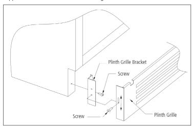
**NOTE**: To be installed with a 150mm plinth height.
