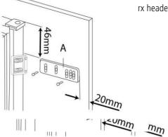
> Clip the door guide cover (part b) on the abor guide (part A) maing the screws.
