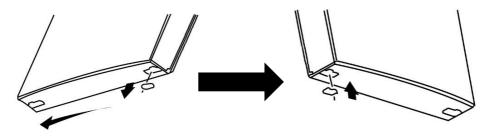
> Flip over the lower hinge 180° and fix on to the opposite side at the bottom of the appliance. Place the door back on to the lower hinge.
