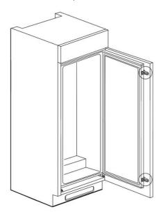
There are 2 hinge covers supplied for the lower and upper hinges. These can be clipped on if required.
