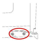
> Remove all of the screw cap covers on the opposite side of the appliance from where the hinges have just been removed. Remove the hinge plugs on the top and bottom of the door and fix them to the opposite side.
