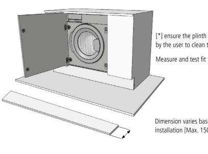
[\*] ensure the plinth can be removed by the user to clean the filter
