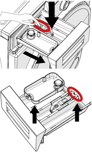
Press the region shown below inside the detergent drawer you have pulled all the way back, and continue pulling and remove the detergent drawer from its place.
