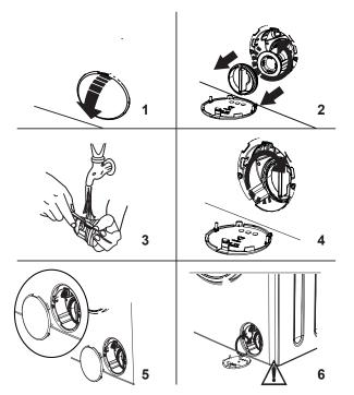
The pump filter system in your Washing Machine prolongs the life of the pump by preventing lint from entering your machine.
