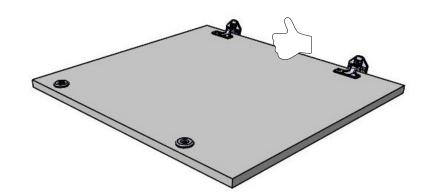
Insert the hinges into the furniture door and use the two wood screws to fix in place.
