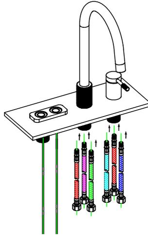
3. Attach the T-piece connector to the Cold mains water supply, to allow a separate flow to go direct to the water filter. The Blue tube supplied with the filter, will need to be cut into 4 appropriate pieces. Connect one piece to the T-piece connector via the push fit connection. The opposite end can then be attached to the inlet on the filter head. The filter comes supplied with a splitter. Using another piece of the blue piping, connect the filter head outlet to the splitter.
