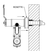
Slide the rosette over the concealed fixing screws until it is flush with mounting surface.
