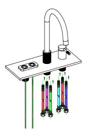
3. Attach the T-piece connector to the Cold mains water supply, to allow a separate flow to go direct to the water filter. The Blue tube supplied with the filter, will need to be cut into 4 appropriate pieces. Connect one piece to the T-piece connecter via the push fit connection. The opposite end can then be attached to the inlet on the filter head. The filter comes supplied with a splitter. Using another piece of the blue piping, connect the filter head outlet to the splitter.
