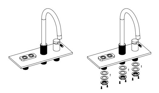
2. Screw the Hot & Cold flexi hoses into the base of the hot/cold handle. The red hose connects to the hot water, the blue hose connects to the cold water. The boiling water flexible hose and the filtered water flexible hose connect to the base of the spout. The handle then needs to be connected to the spout via the additional flexi hose, as shown in the diagram here:
