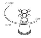
The side spray uses a sequential cartridge. This means that you will have cold, tepid and hot water, in this order, once you start opening the tap
