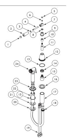
The set comprises of the following: ITEM QTY DESCRIPTION 1 Ceramic Handle Nut 2 Ceramic Handle 3 O-Ring 1 4 Handle Stem 5 Indicie 6 Screw 7 Handle 1 8 Handle Ring 9 Handle Cover 10 Washer 11 Handle Extension 12 Cartridge Cover 13 O-Ring 2 14 Nut 1 15 Progressive Cartridge 16 Locking Nut 17 Cartridge Body 18 Spray Hose 19 Connection 20 Locking Nut 21 Washer 22 Handset Holder 23 Holder Plate Spray Handset 24
