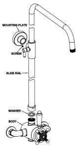
Step 7: Apply washer into the bottom of sliding rail then fix the sliding rail onto the mixer body. Then fix sliding rail onto mounting plate, tighten with screw.
