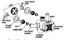
Step4: Place the components and body as per the order above. Turn nuts on the body, then fix the mixer onto the wall with locking screws, tighten the nuts with spanner to seal.
