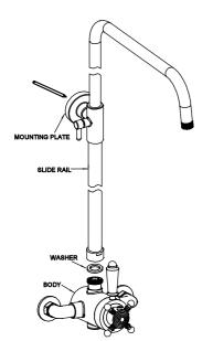
Step 5: Apply washer into the bottom of sliding rail, then fix the sliding rail onto the mixer body. Make markings for the position of the mounting plate, then take off the sliding rail.
