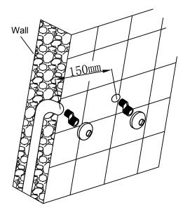
2.Fix the shower valve to the off-set connector using a spanner. Please use a cotton sheet inside of spanner to avoid any scratches. Make sure hot outlet is on the left and the cold outlet is on the right, otherwise it will affect the performance.
