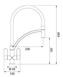
The Zelus is a stunning tap with coloured hose and pull-out nozzle with perlator - also available in Chrome or SilkSteel Spring Hose versions. Features rounded paddle handles.
