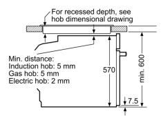
measurements in mm
