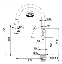
With the Pescara Swivel Up Down tap, the water flow changes by a simple up/down motion at the end of the spout.
