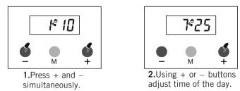
**Note:** Unless the + or – buttons are pushed along 5 seconds, time of the adjustment mode will be end up automatically. If you want to finish time of the adjustment mode rapidly, you should press + and – buttons simultaneously.
