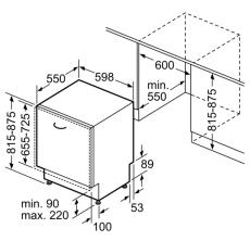
measurements in mm
