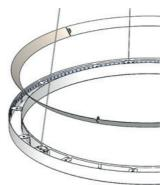
Carefully remove the LED bar. Disconnect the connector and change the LED light.
