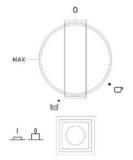
The control elements are the temperature knob and the luminous ON-OFF switch. With the switch pressed (position 1) the drawer is on, whereas when the switch is released (position 0) the drawer is off. These parts can be seen only when the drawer is open. When the drawer is closed, a control light located on the front of the appliance lets you see whether the drawer is on.
