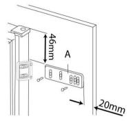
> Clip the door guide cover (part B) on the door guide (part A) hiding the screws.
