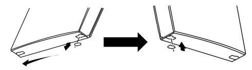
> Flip over the lower hinge 180° and fix on to the opposite side at the bottom of the appliance. Place the door back on to the lower hinge.
