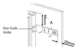
> If any adjustment is needed use the clearance space in the screw slots of the door guide holder on to the door guide (part A).
