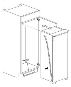
> Open the door and push the side of the appliance without the hinges against the side of the cabinet wall. Fix the appliance in 2 places, 2 torx headed screws in the top plinth at the top of the appliance and 2 torx screws in the feet (1 in each foot) at the bottom of the appliance.
