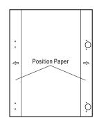
Cut door template paper Paste on the door (the door on the right)
