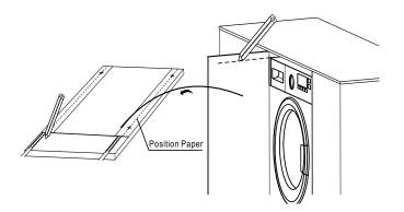
2. Fix door template onto the door.
