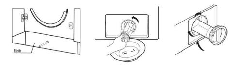
**WARNING:** The filter must be cleaned periodically to ensure the normal operation of the washing machine.
