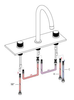
3. Attach the T-piece connector to the Cold mains water supply, to allow a seperate flow to go direct to the water filter. Using the Blue tube supplied with the filter, cut it to the appropriate length and connect this to the T-piece connecter via the push fit connection. The opposite end can then be attached to the inlet on the filter head.
