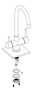
2. Screw the 3 flexible hoses into the base of the tap. The red hose connects to the hot water, the blue hose connects to the cold water, and the longer plain steel hose (1 meter) connects to the boiling water.
