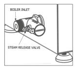
7. The clear silicone hose connects to the steam release valve on the side of the boiler, and can then be attached to the existing plumbing using the threaded metal connector.
