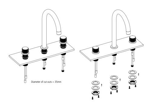
2. Screw the Hot & Cold flexi hoses into the base of the hot & cold handle. The red hose connects to the hot water, the blue hose connects to the cold water. The boiling water flexible hose connects to the base of the boiling water handle. Each handle then needs to be connected to the spout via the additional flexi hoses, as shown in the diagram here:
