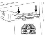
**2.** To return the heating element to its position, lift it up, pull it slightly towards you and make sure that the tab support is in its proper seating.
