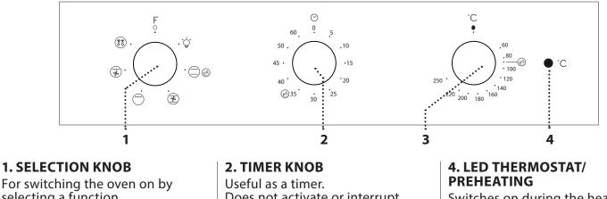
For switching the oven on by selecting a function. Turn to the position O to switch the oven off.
