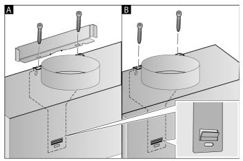
5. If no duct is to be fitted, screw in the two locking screws without the bracket. **B**
