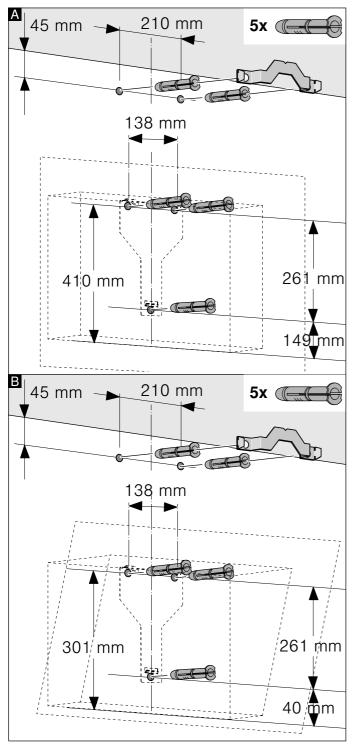
Fitting without a flue duct
