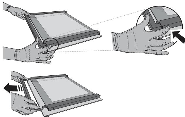
**2.** Lift and firmly hold the inner glass with both hands, remove it and place it on a soft surface before cleaning it.
