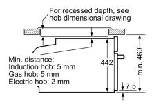
measurements in mm
