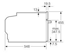
measurements in mm
