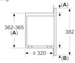
A: Overhang at top: Recess 362: 6 mm Recess 365: 3 mm B: Overhang at bottom: 14 mm
