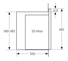
measurements in mm
