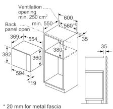
measurements in mm
