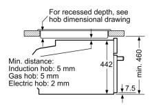
measurements in mm
