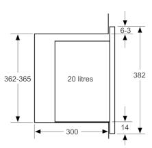
measurements in mm
