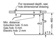
measurements in mm
