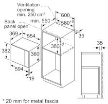
measurements in mm
