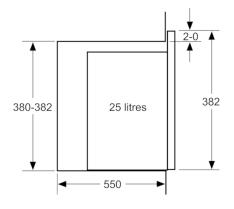
measurements in mm
