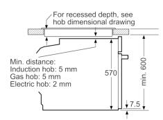
measurements in mm
