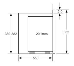
measurements in mm
