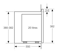
measurements in mm
