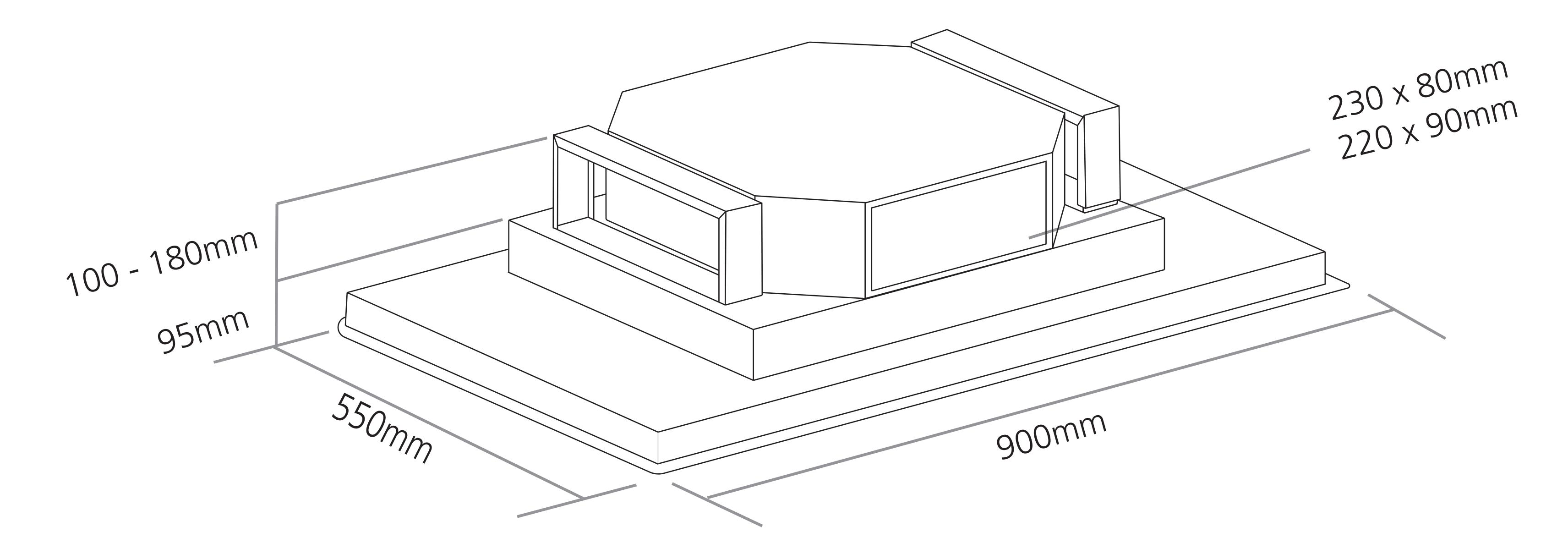
For the installation, create a false ceiling with a niche of 865mm for 515mm whose minimum height to be reached is 200 mm
