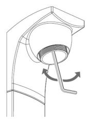
**4.** Using a 3mm hexagonal key turn the flow screw clockwise for a longer flow time and anti-clockwise for a shorter flow time.
