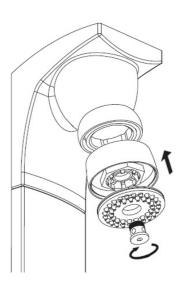
**6.** Push the spray plate holder and spray plate onto the locking collar and secure in position by tightening The locking screw.
