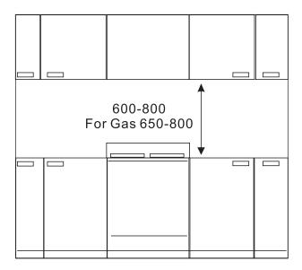
Pictures: Minimum height from the hob surface to the underside face of the rangehood is : 600mm for electric hob, 650mm for gas hob.
