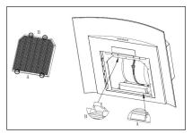
After assembly, the charcoal filter should be as below:
