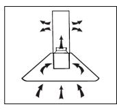
If you do not have an outlet to the outside, the exhaust pipe is not required (as shown in the section "Installation - ducted"), and charcoal filters must be installed.
