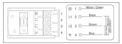
If the total number of heating units of the appliance you choose is not less than 4, the appliance can be connected directly to the mains by single-phase electrical connection, as shown below.
