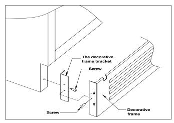
Note: To be installed with a 150mm plinth height.
