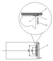
After installing the wine cabinet, please open the door, adjust the fixing bracket (a) and fix this in position with three screws (c) using a screwdriver (d) into the work surface.
