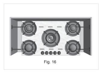
**4a.** The PITT<sup>®</sup> cooking module should always be fully supported with the PITT<sup>®</sup> cooking support set to prevent bending of the kitchen worktop (**fig. 15 and 16**).
