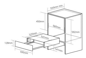
See below for an example of the WD140BK installed below the 45cm Steam oven (SO110):
