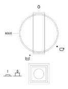
The control elements are the temperature knob and the luminous ON-OFF switch. With the switch pressed (position 1) the drawer is on, whereas when the switch is released (position 0) the drawer is off. These parts can be seen only when the drawer is open. When the drawer is closed, a control light located on the front of the appliance lets you see whether the drawer is on.
