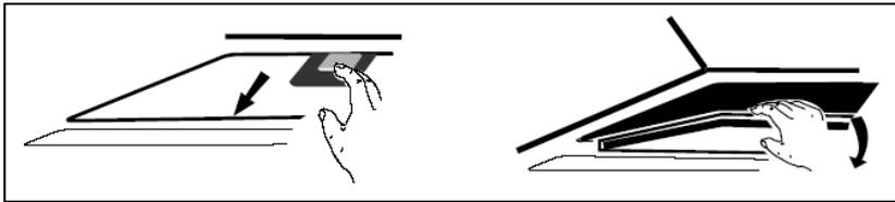
To fit the charcoal filter, line up part A of the charcoal filter with the rear bar, and part B of the filter with the front of the hood. Push the filter into this space to secure it. There are 2 clips on part B which lock the filter into place once it has been pushed in.
