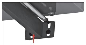
6. Push the beams firmly against the underside of the PITT<sup>®</sup> cooking unit and tighten the upper two screws completely. Then, tighten the lower screws completely.
