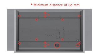
4. Position the beams in such a way that the screws, gas connection and the electricity block are freely accessible.
