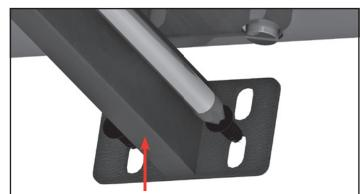
5. Push the beams firmly against the underside of the PITT<sup>®</sup> cooking unit and tighten the lower two screws by hand. Repeat this step for the other side of the cabinet.
