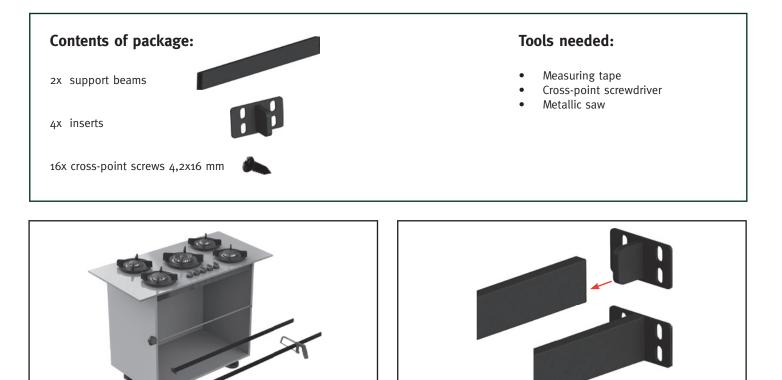
2. Place the inserts into the ends of the beams that have been cut to size.
