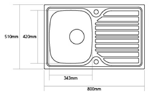
Bowl Depth 150mm Min. base unit 450mm Cut out size 776 x 486m
