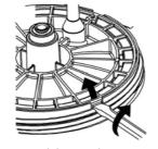
8. Lever lid upwards using screwdriver under 3 x lugs.
