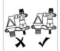
Connect drain valve assembly (E3) to the hot water hose (D1) ensuring fibre seal (D2) is in place.
