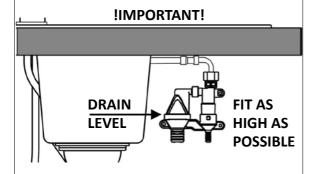
The drain valve (E3) needs to be fitted as high as possible. This is to help prevent the possibility of a blocked sink flowing out to the drain valve (E3).
