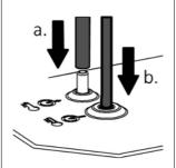
17. Push rubber hose (a) and pipe (b) fully onto stems as shown. Return unit to former position.
