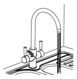
18. Turn on until water runs through spout, then fully turn off.
