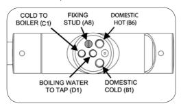
This diagram shows the markings on boiler (E1) to indicate the inlet and outlet. See the boiler instructions for further detail.
