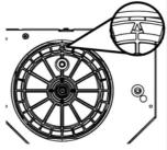
11. Replace tank lid, ensure arrow is to rear as shown.
