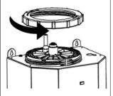
7. Unscrew tank lid ring anticlockwise.
