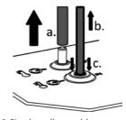
Firmly pull up rubber hose (a) collar (c) down and pull pipe (b) out simultaneously. Prepare for small spillage. Remove to bench (if desired)
