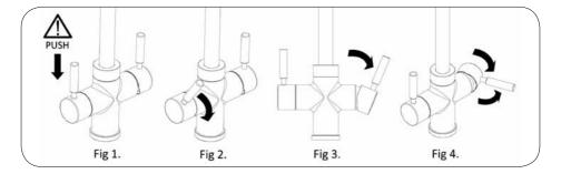
A Should you see that hot water persistently drips from the centre channel of the tap spout (when the tap is not in use and the boiler indicator red light is switched on) then you should reduce the temperature adjustment dial on the top of the boiler. See the calibration procedure for further information.
