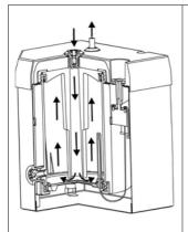
This boiler works on displacement i.e. the cold water is fed into the bottom of the tank which then forces the hot water out of the top. The water temperature is controlled via thermostat. The setting of this is designed to allow the user to set the highest temperature while not allowing the unit to boil continuously.
