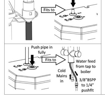
Connect the hot tube (D1) from the drain valve (E3) to the hot outlet of boiler. The pipe needs to be a smooth run with no kinks or sharp bends, the tube can be cut to suit your particular installation.
