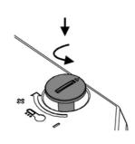
16. Loosely rotate temperature knob until it drops then press down.
